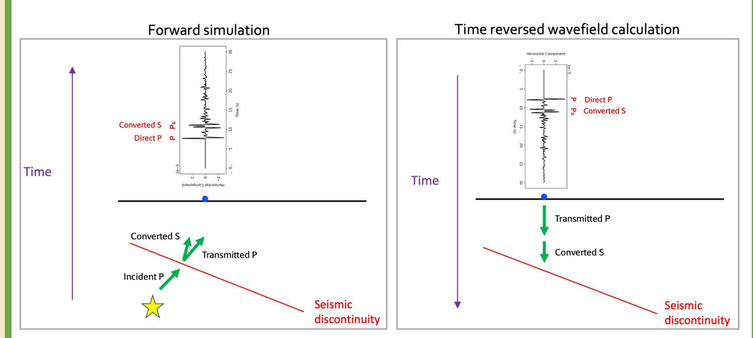
Prior attempts to formalize converted wave imaging have had issues with SNR. We overcome these issues through (1) increasing signal amplitude by cross correlating only the components of direct P and converted S that are expected to have large amplitudes and (2) decreasing artifacts by windowing seismic data prior to backpropagation to prevent undesired interference from other seismic phases. We also normalize by the ray parameter to remove dependence on the seismic wavefield.
