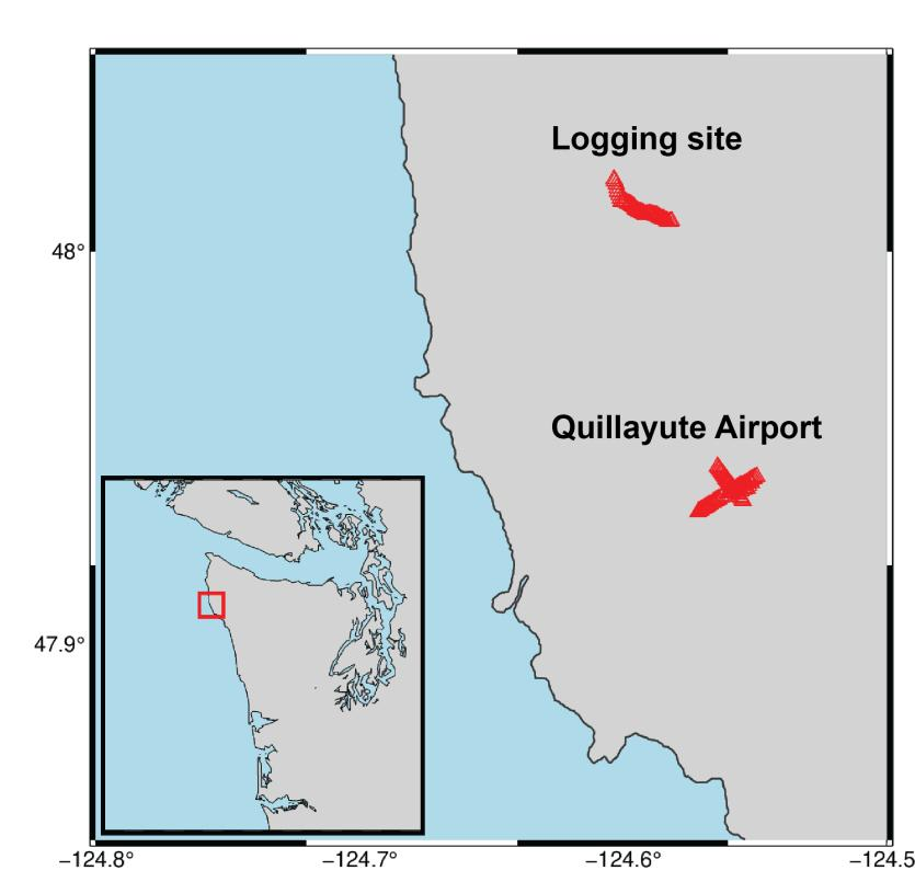
98 seismic nodes were deployed near Forks, WA from August 2021 - December 2021. This location was chosen because the locked zone comes onshore here and there is local seismicity at depths below the overriding plate. The seismometers were deployed at a logging site and at the Quillayute Airport.
