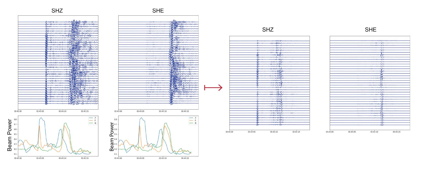
These record sections show data collected by our arrays during a M2.2 earthquake that occurred at 29km depth in Oregon on August 31, 2021. The upper panel on the left shows the original data. The panels on the right show seismograms that have been windowed using the beam power to isolate the phases of interest so that we can produce clean backpropagated wavefields.
