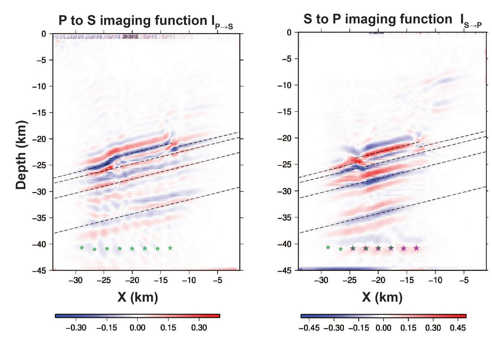
Our method successfully recovers all of the important boundaries in the subduction zone structure using either Ps or Sp converted waves.
