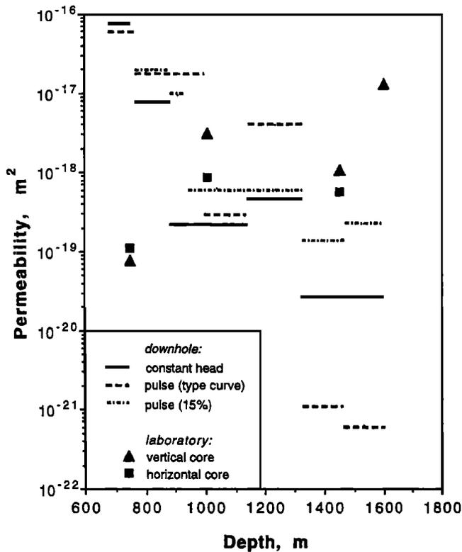
**Figure 2.** Permeability (from Figure 1) of core samples at estimated in situ effective pressures (closed symbols, this study) and downhole permeability determined from constant head and pulse flow tests for selected depth intervals (solid or dashed lines, modified from *Haimson and Doe* [1983]). See *Haimson and Doe* [1983] for a discussion of uncertainty errors for the three types of downhole flow tests.
