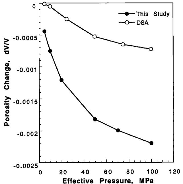
Figure 5. Comparison of porosity change (this study) and volumetric crack strain (from Differential Strain Analysis data, Kowallis and Wang [1983]) as a function of effective pressure for the 751.3H-m sample.
