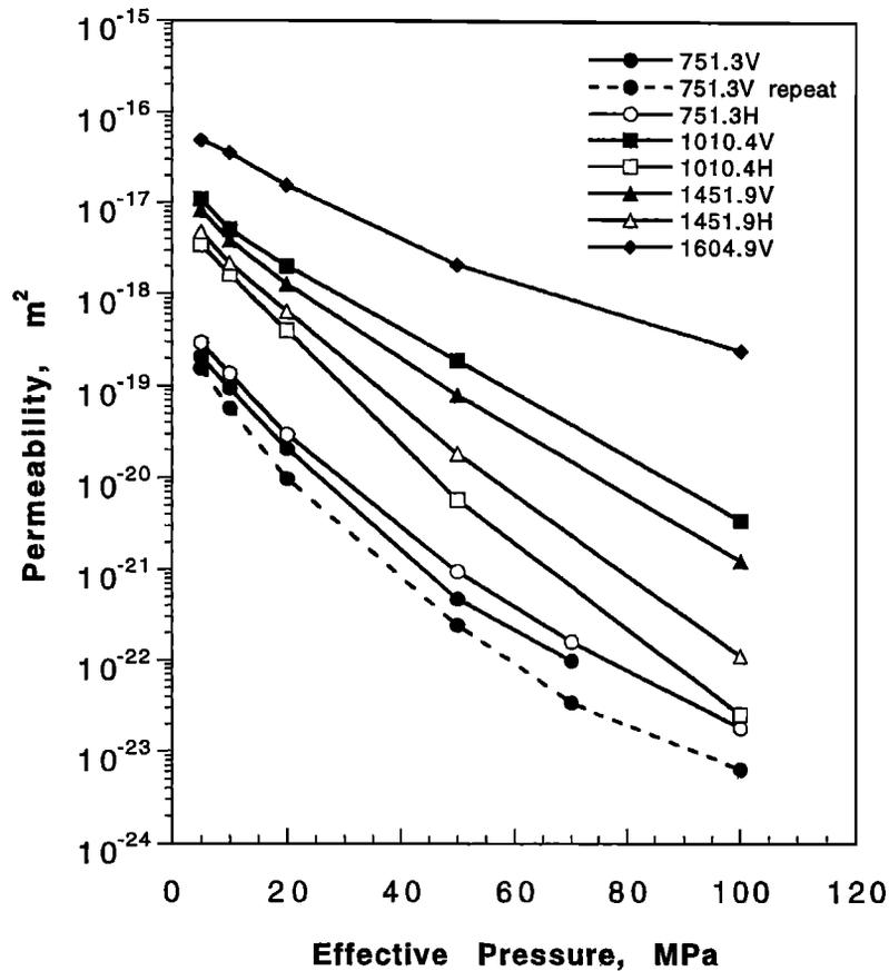
Figure 1. Permeability of Illinois UPH 3 drillhole samples as a function of effective pressure. Sample depth in meters for vertical (V) and horizontal (H) cores.
