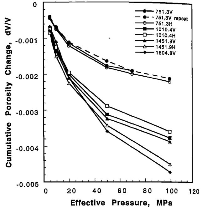
**Figure 3.** Cumulative porosity change of Illinois UPH 3 core samples as a function of effective pressure. Sample depths in meters.
