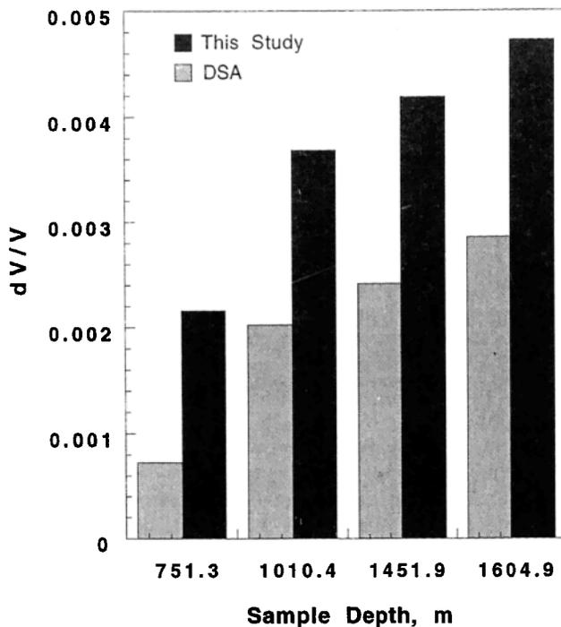
Figure 6. Comparison of volumetric crack porosity at 100 MPa, vertical and horizontal samples (this study) averaged. Differential Strain Analysis data from Carlson and Wang [1986].
