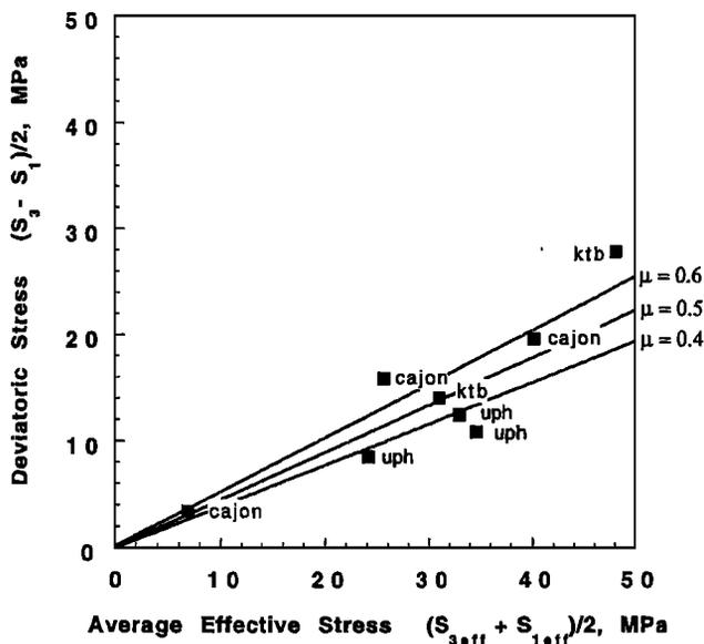
Figure 7. Deviatoric and average effective stress from downhole measurements at the Cajon Pass (California), KTB (Germany) and UPH 3 (Illinois) drillholes. In situ stress data [Zoback and Healy, 1992; Zoback et al., 1993; Haimson and Doe, 1983] chosen at depths from which we also have laboratory permeability measurements on core samples. Lines show coefficient of friction envelopes for  $\mu = 0.4, 0.5, \text{ and } 0.6$ .
