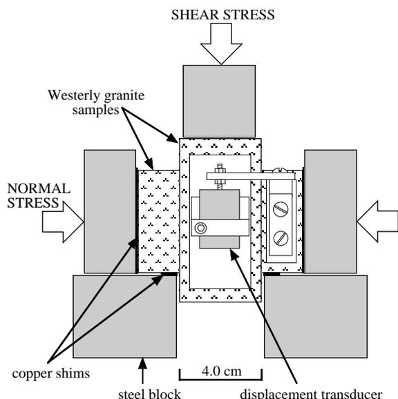
Fig. 2. The three block, sandwich-type direct shear sample configuration used in these experiments.
