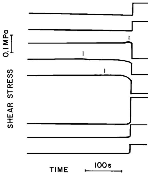
Fig. 3. Confined unstable slip event. Curves give shear stress at equal intervals along the sliding surfaces. The vertical lines indicate the time of onset of premonitory fault slip.
