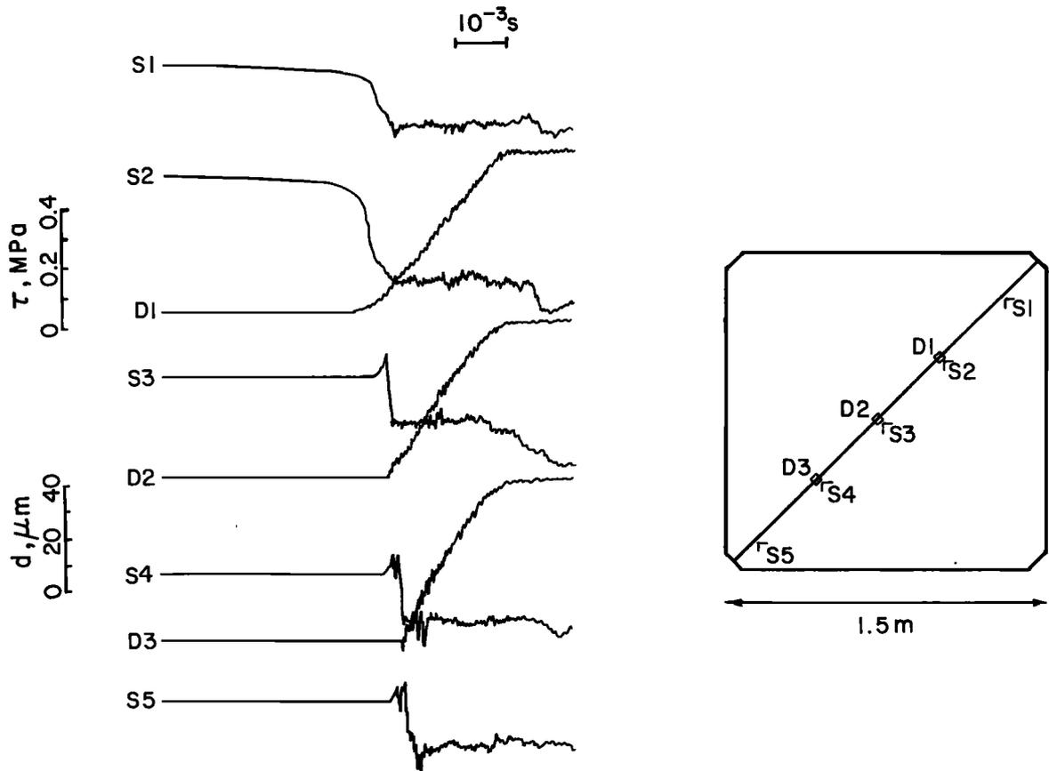
Fig. 2. Details of unstable slip event. Curves D1-D3 give fault displacement and curves S1-S5 give the component shear stress parallel to the fault.
