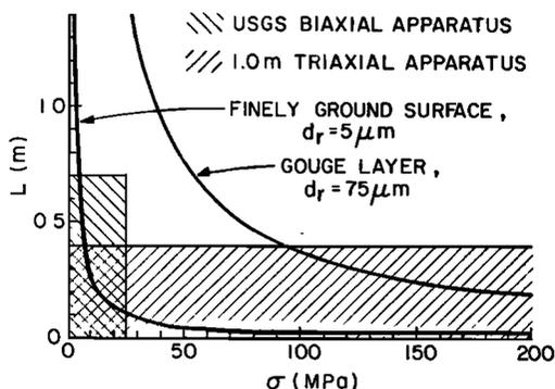
Fig. 4. Predicted minimum dimension for confined unstable slip ( $L$ ) plotted against normal stress ( $\sigma$ ) for a finely ground surface ( $d_r = 5\mu\text{m}$ ) and a fault with fine gouge ( $d_r = 75\mu\text{m}$ ). Cross-hatched areas give the approximate operating range of the biaxial apparatus described here and a hypothetical triaxial apparatus.
