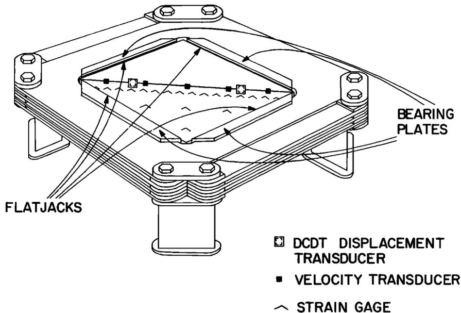
Fig. 1. Diagram of apparatus.
