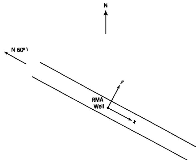
Fig. 5. Plan view of infinite strip reservoir used for analysis.
