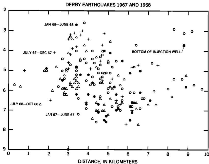
Fig. 3. Northwest-southeast cross section on which are plotted the earthquakes reported by Hoover and Dietrich [1969] for 1967 and 1968.
