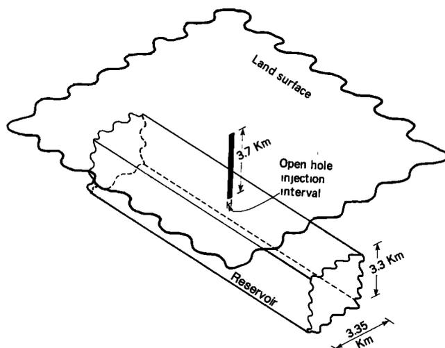
Fig. 4. Oblique view of the idealized reservoir modeled as a long, narrow prism of isotropic, porous medium.
