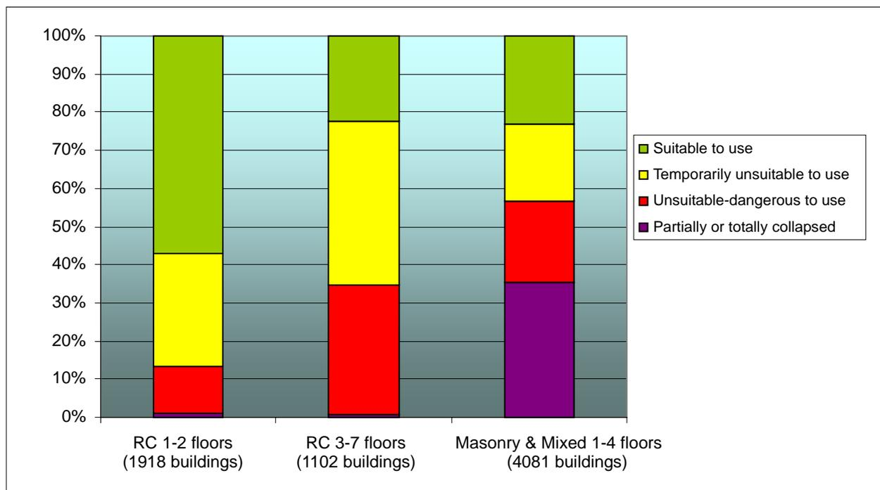
Figure 2 Damage distribution in the city of Kalamata following the 1986 earthquake
