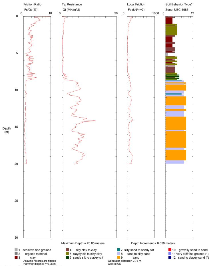
Hammer distance = 0.96 m Soil behavior type and SPT based on data from UBC-1983\*
