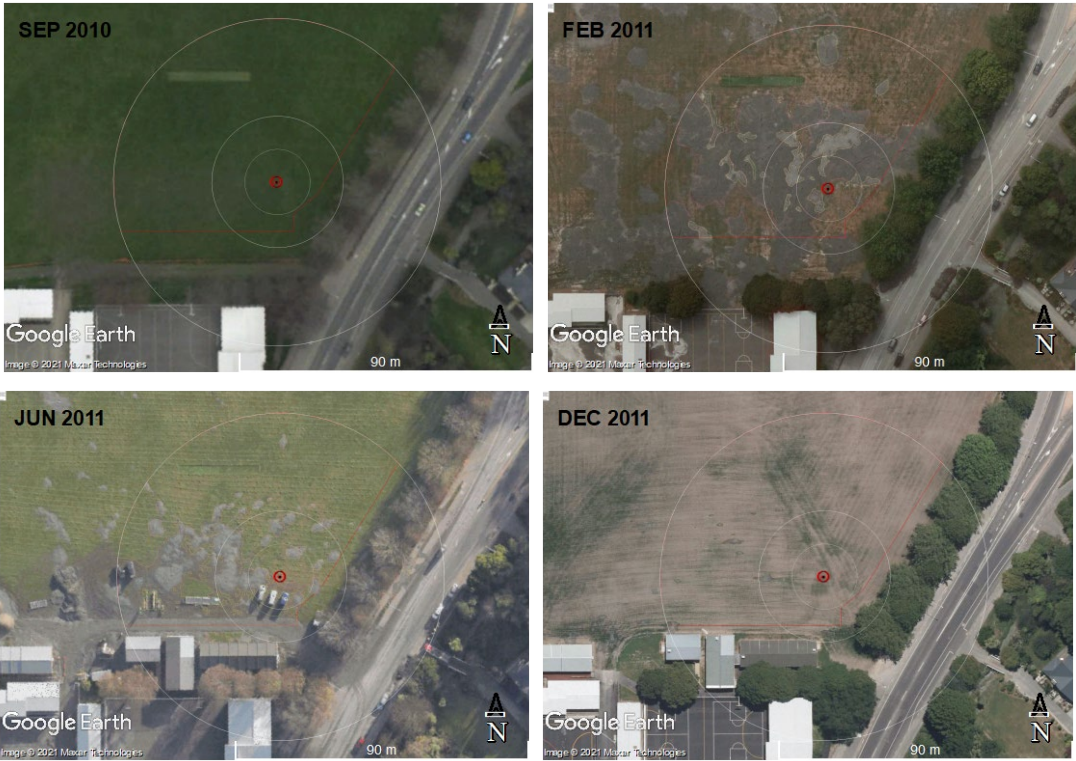
Figure 9: Aerial photographs acquired for Shirley Intermediate School in Sep 2010, Feb 2011, June 2011, and Dec 2011 (CGD 2012a) with ejecta outlines for the 10-, 20-, and 50-m buffers.
