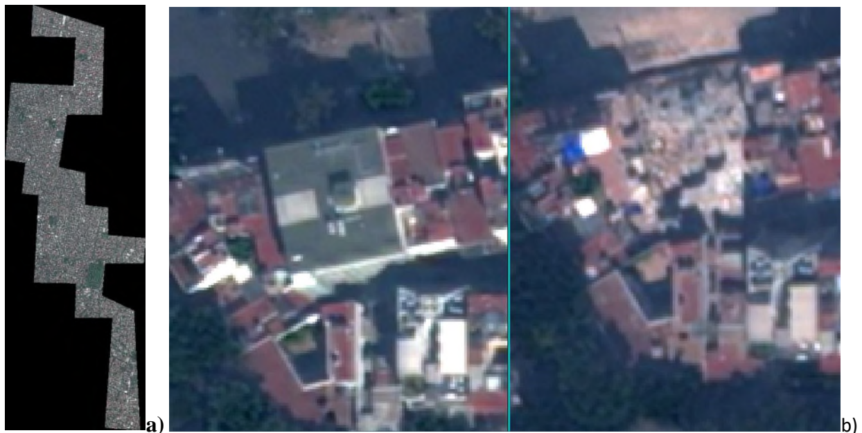
Figure 2. a. World-View 2 imagery from October 20, 2017 capturing collapsed and intact buildings after the September 19, 2017 Mexico Earthquake. b. zoom of collapsed and intact buildings shown pre-event (left) and post-event (right).
