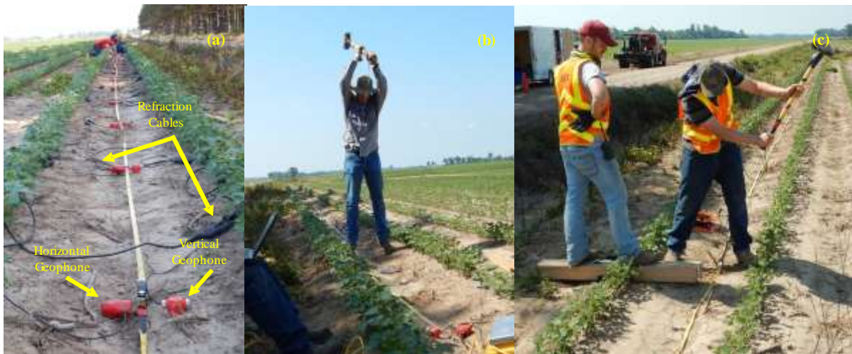
Figure 5. A general testing methodology for MASW and P-wave refraction is shown. In (a), linear array of vertical and horizontal geophones is shown. In (b) and (c), Rayleigh and Love wave generation, respectively from vertical and horizontal sledgehammer impacts are shown.
