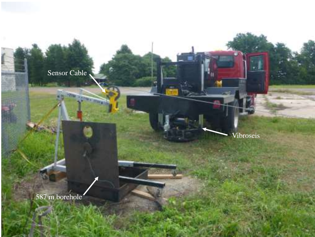
Figure 8: Deep downhole equipment layout for CUSSO site at 587 m borehole.
