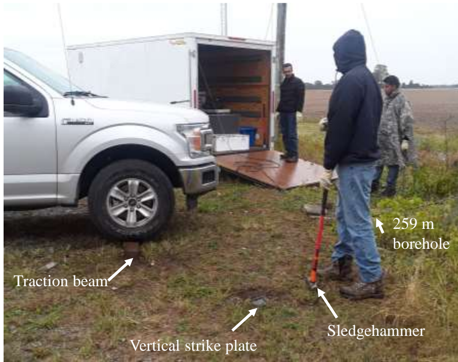
Figure 7: Shallow downhole equipment layout for CUSSO site at 259 m borehole.
