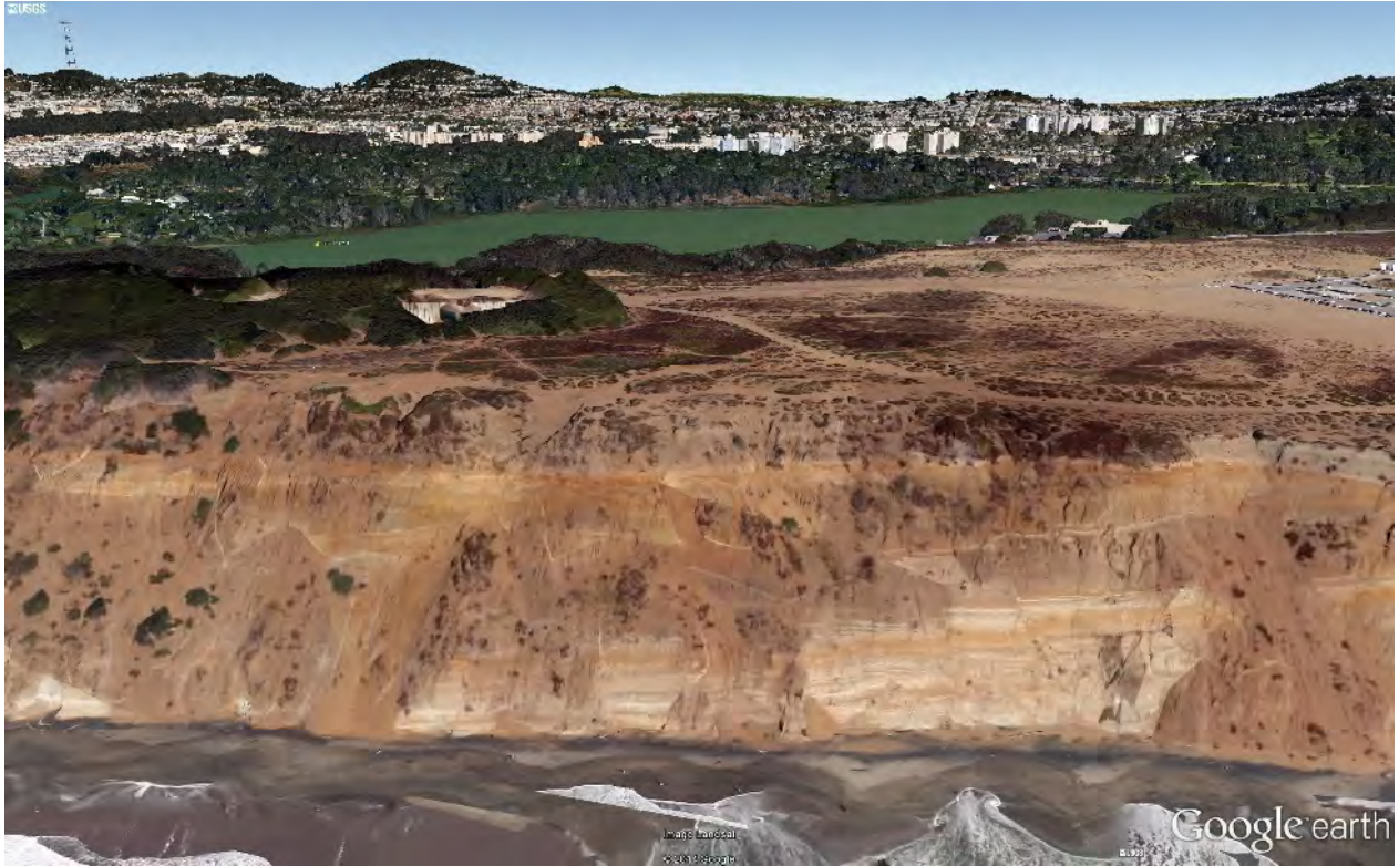
Figure 7. Google Earth view across Thornton beach and the exposed ~ 60 m cliffs with NE dipping Merced (lower) and Colma formations (upper). Lake Merced, San Francisco and Sutro Tower on the skyline. (The high resolution photos have numerous overlap artifacts).
