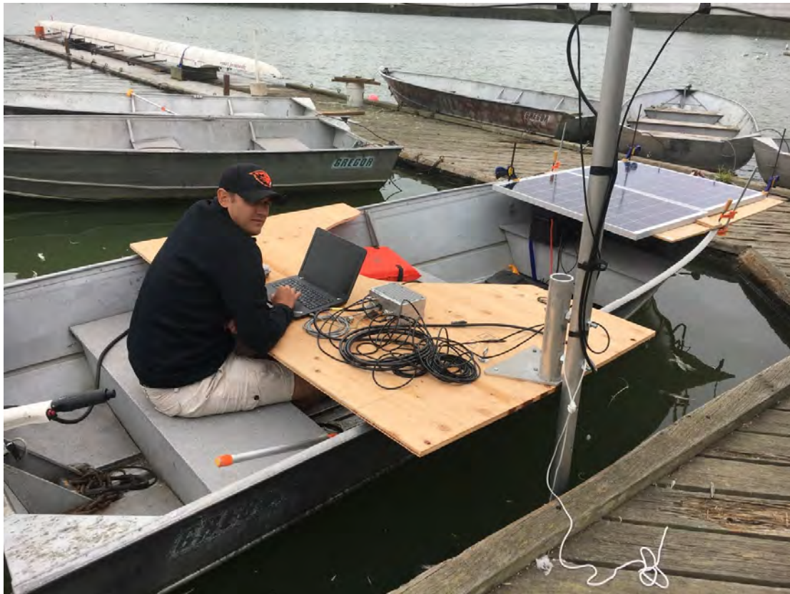
Figure 15. Survey vessel used for Lake Merced. Knudsen Engineering 3-20 kHz CHIRP subbottom profiler and Norbit broadband multibeam sonar were mounted on starboard pole mount. Upper part of pole carried dual GPS sensors for the motion sensing unit. Boats, motors and facilities kindly provided by the Pacific Rowing Club, Jeff Beeson pictured.
