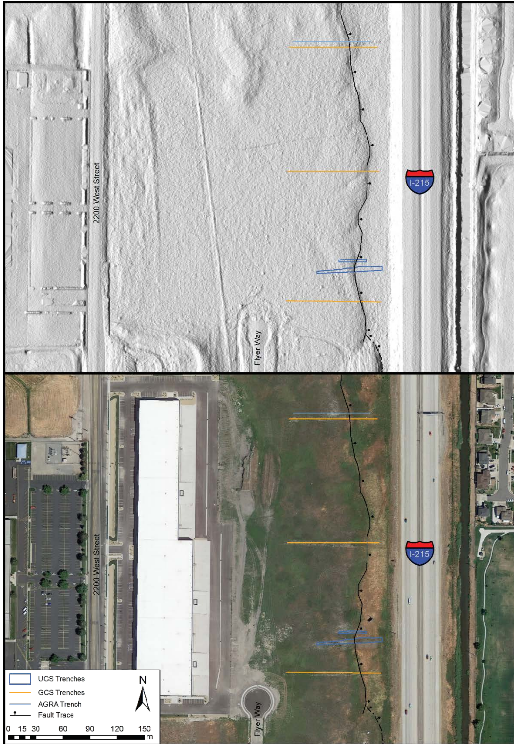
Figure 4. Overview of the Airport East site and vicinity; lidar hillshade image (top) and orthophoto (bottom). Bar-and-ball symbols on downthrown side of fault. Previous trench locations are approximate; AGRA trench was excavated in September 1997, GCS trenches were excavated in August 2014. Lidar: 0.5-m posting, hillshade illumination from the west (Utah Automated Geographic Reference Center, 2014). Orthophoto: Google Imagery, 2016.
