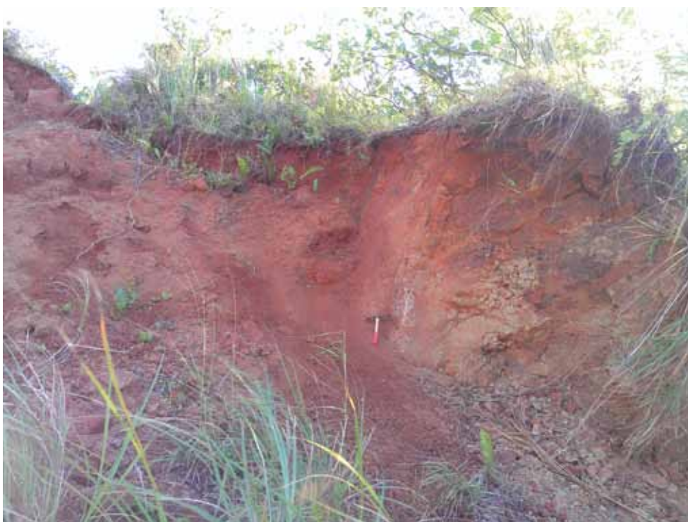
B. Faulting in Alutom Fm. with unfaulted overlying alluvium at Site M2
