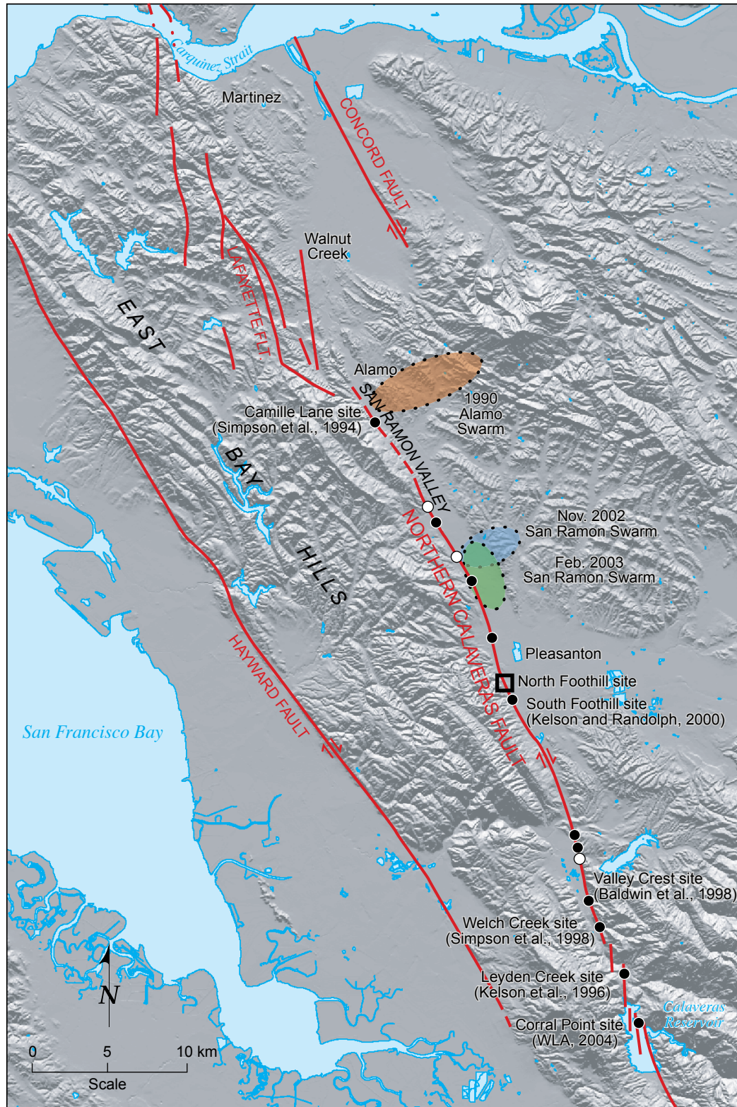
Regional map of the Northern Calaveras fault showing previous paleoseismic sites (filled circles), creep observation sites (open circles), and this study site (open square). Faults northwest of Alamo are from Unruh and Kelson (2002).
