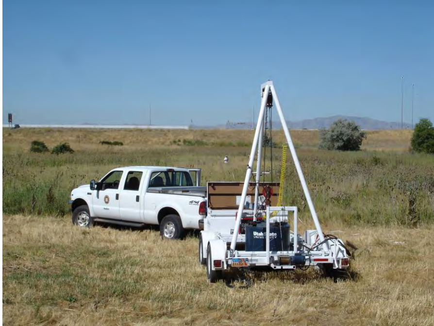
Fig. 2.120 Photograph of SASW testing at the Utah Highway Patrol Building (UHP), Davis County, Utah.
