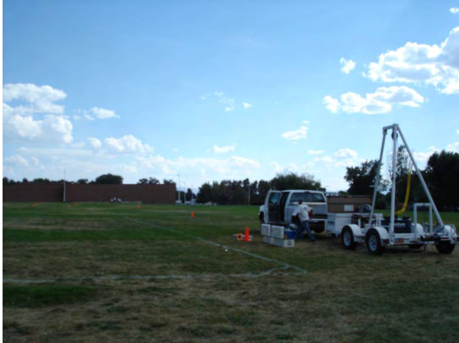
Fig. 2.228 Photograph of SASW testing at Pleasant Grove Junior High School (PJH), Utah County, Utah.
