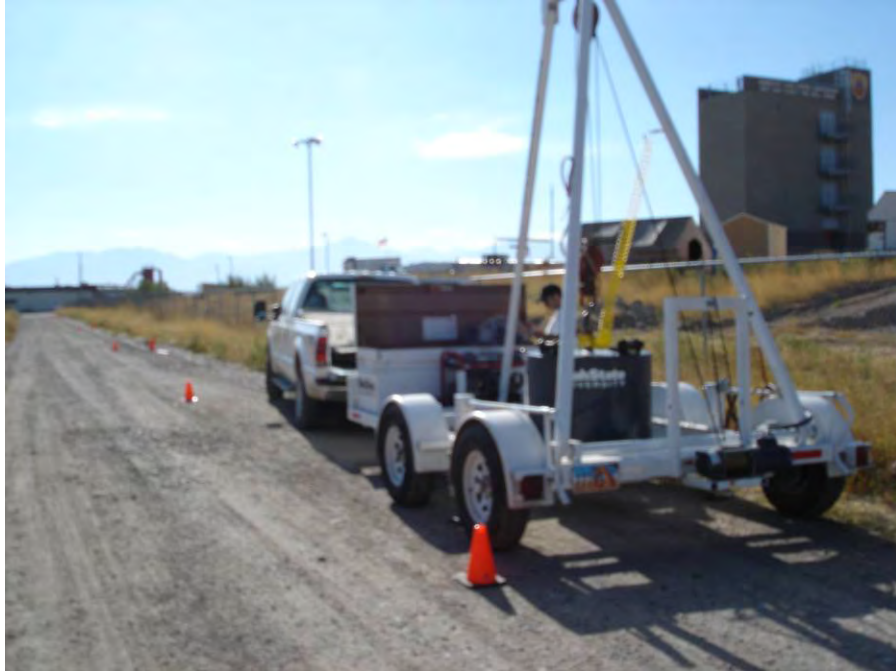
Fig. 2.141 Photograph of SASW testing at the Fire Training Tower (FTT), Salt Lake County, Utah.
