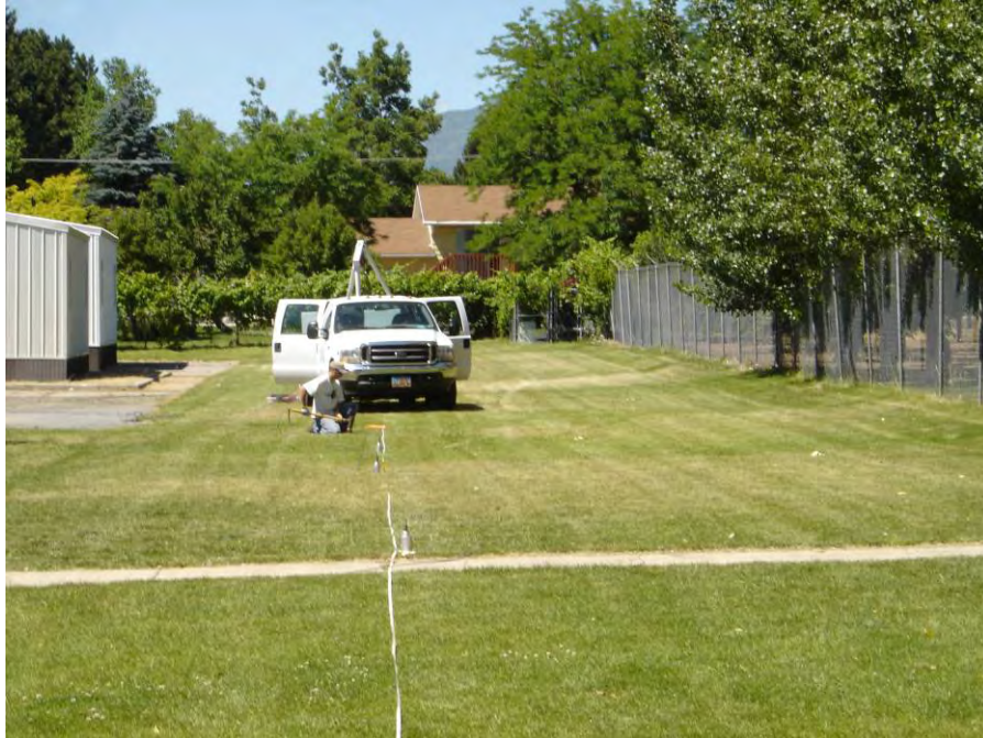
Fig. 2.33 Photograph of SASW testing at East Layton Elementary School (ELE), Davis County, Utah.
