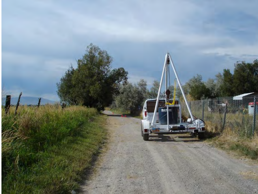
Fig. 2.178 Photograph of SASW testing at the Salem City Yard (SCY), Utah County, Utah.
