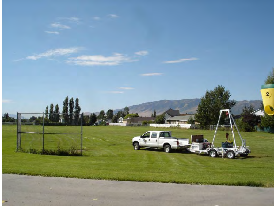
Fig. 2.163 Photograph of SASW testing at the Meadow School (MDS), Utah County, Utah.
