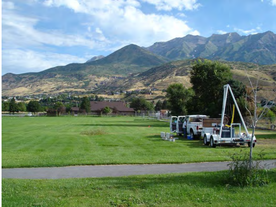
Fig. 2.223 Photograph of SASW testing at Orchard Elementary School (OES), Utah County, Utah.
