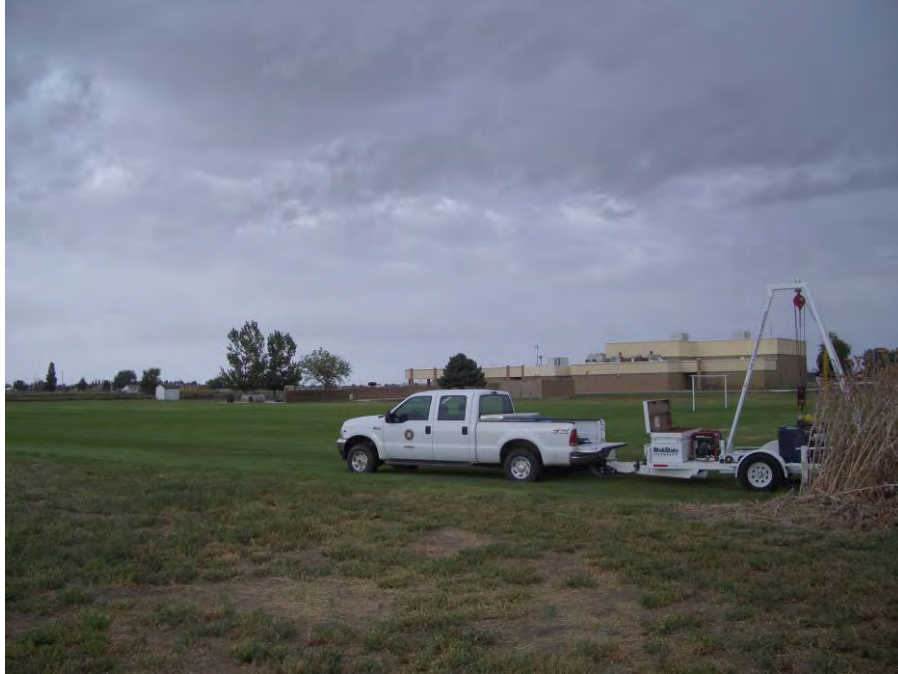
Fig. 2.18 Photograph of SASW testing at Kanesville Elementary School (KSU), Weber County, Utah.
