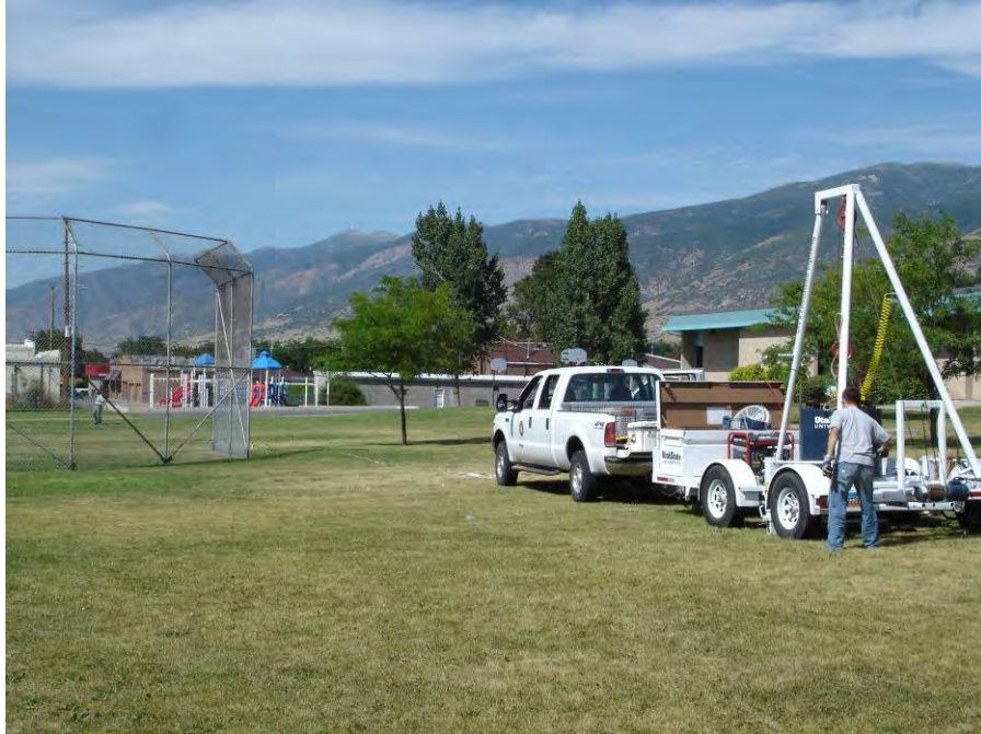
Fig. 2.115 Photograph of SASW testing at Washington Elementary School (WSE), Davis County, Utah.
