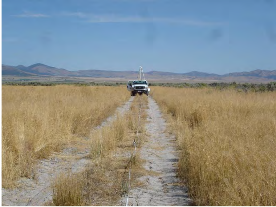
Fig. 2.203 Photograph of SASW testing West of Utah Lake (WUL), Utah County, Utah.
