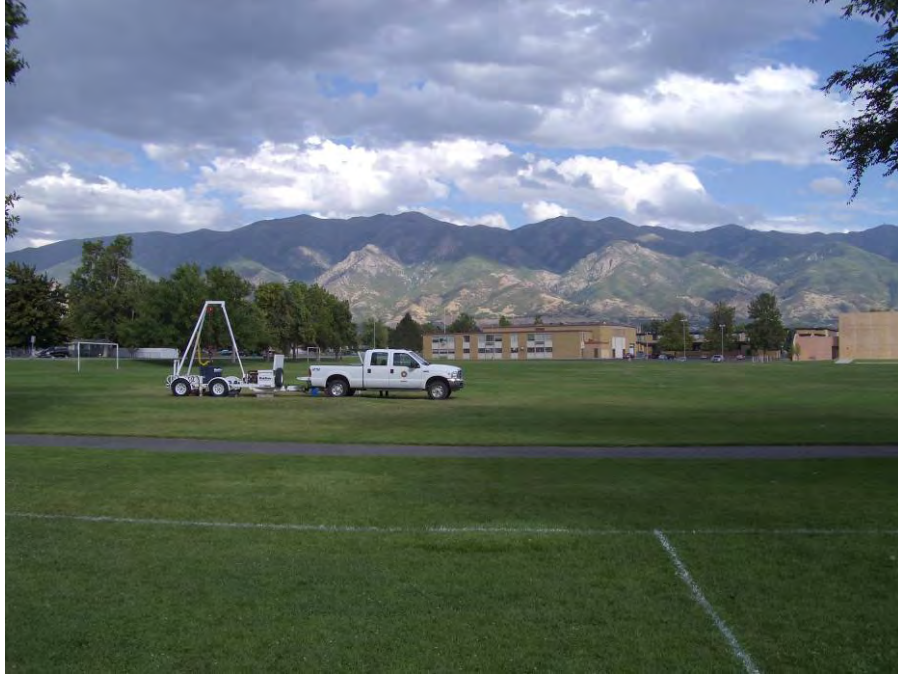
Fig. 2.13 Photograph of SASW testing at Central Davis Junior High School (CDJ), Davis County, Utah.
