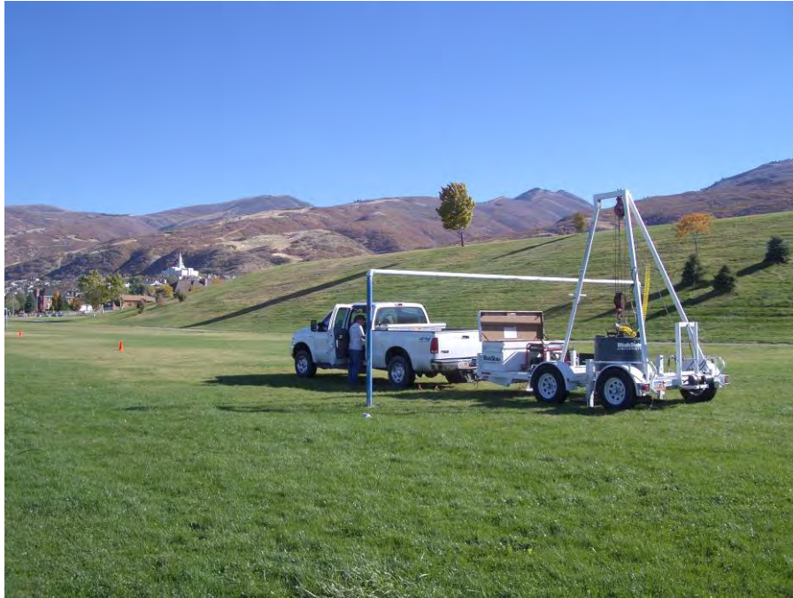
Fig. 2.135 Photograph of SASW testing at Mueller Park Junior High School (MPS), Davis County, Utah.
