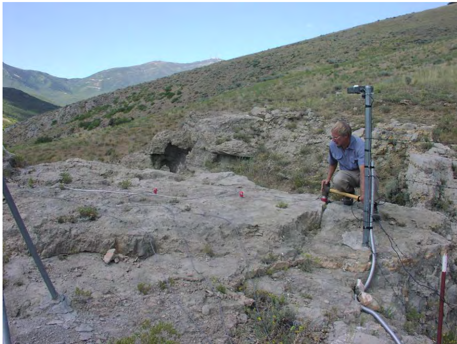
Fig. 2.148 Photograph of SASW testing on the rock site at the North Oquirrh Seismic Station (NOQ), Salt Lake County, Utah.
