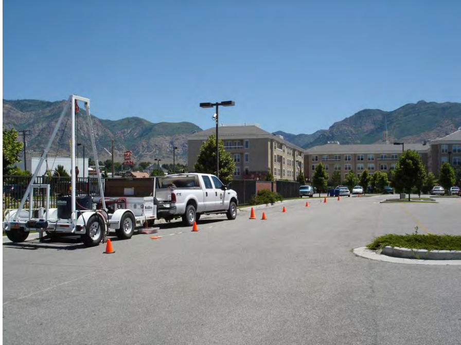
Fig. 2.43 Photograph of SASW testing at the Ogden Public Safety Building (OPS), Weber County, Utah.
