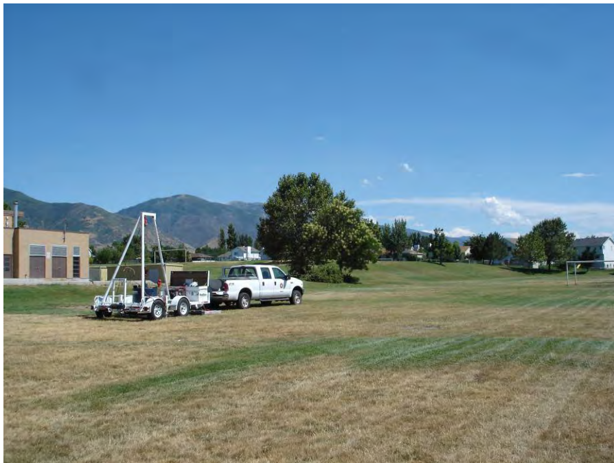
Fig. 2.105 Photograph of SASW testing at Kaysville Junior High (KJH), Davis County, Utah.
