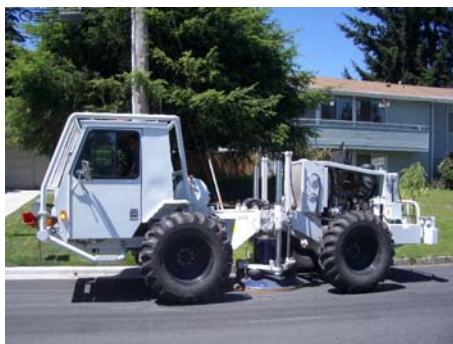
Figure 4. Minivib II truck used during this seismic survey.
