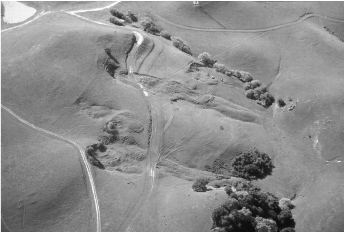
Figure 4.18 Earthflows occupying the axes and flanks of colluvial-filled bedrock ravines near El Sobrante, CA, imaged in January 1993. Earth flows on Crowley's Ridge exhibit the same topographic expression, but are more difficult to visualize on aerial photographs due to the dense vegetation.
