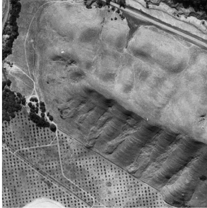
Figure 4.4 – Vertical photo of Campolindo Ridge in Moraga, CA, taken in 1946 with oblique backlighting, which shows a series of dormant earthflows to good effect.
