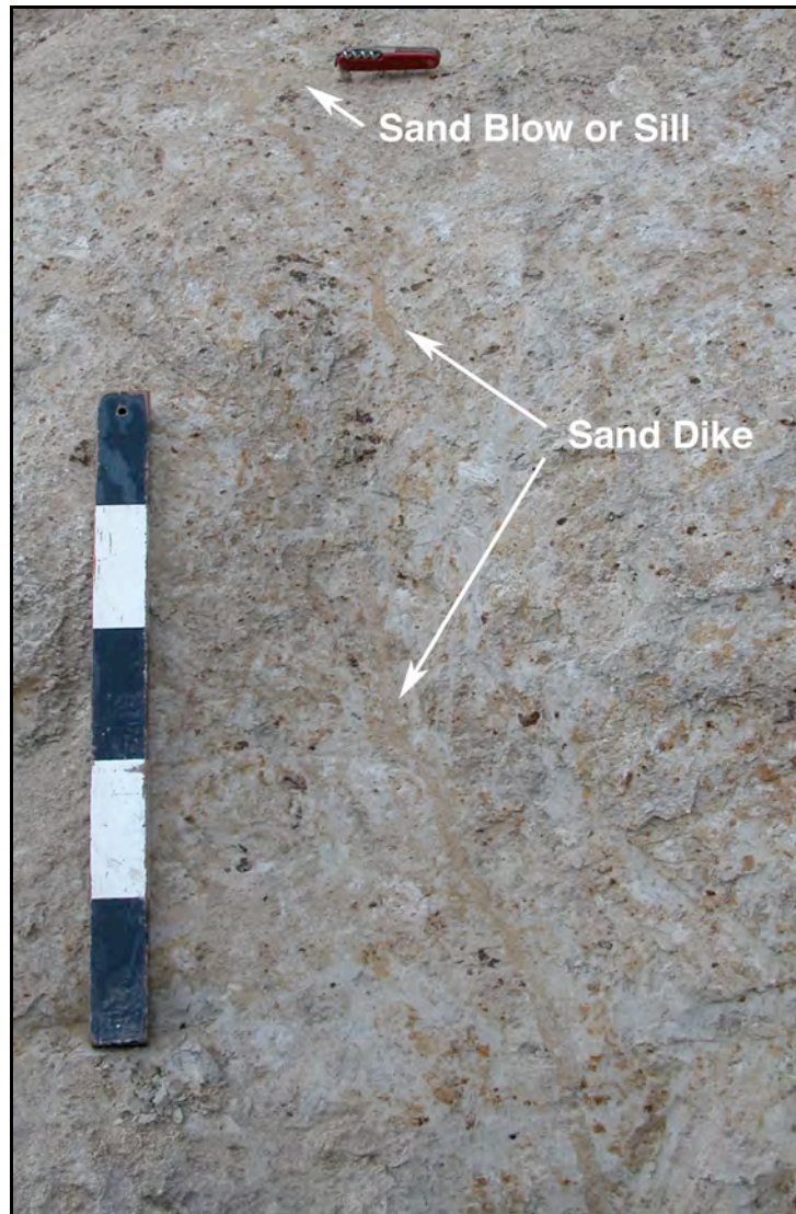
Figure 2. Small liquefaction features, including 1.5-cm-wide sand dike and possible 0.5-cm-thick sand blow or sill at site 38 along Hatchie River. Silt coatings on sand grains and manganese nodules within sand dike suggest that liquefaction features could be thousands of years old. On scale, black and white intervals represent 10 cm.
