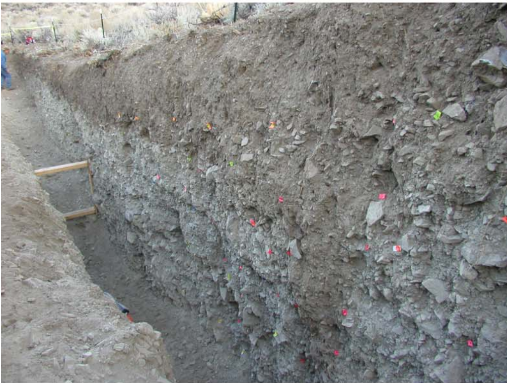
Figure 9. Trench 1, Peavine Peak fault. Dark upper unit and fissure fill is mollic soil that thickens against the fault in response to MRE. Photo by C. dePolo
