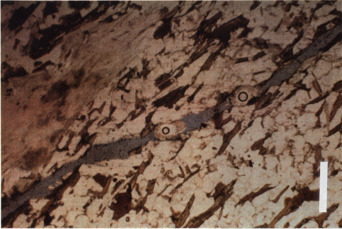
Fig. 2. Optical micrograph of shear fracture in Bi Gneiss shortened at 45°S; scale bar 1 mm. Note feather-type axial microcracks associated with the fracture.
